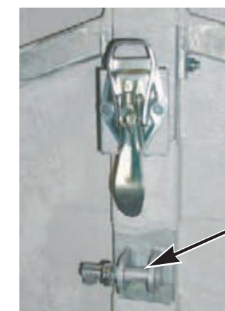
Fig. 68 Bolt for prop on nacelle wall
