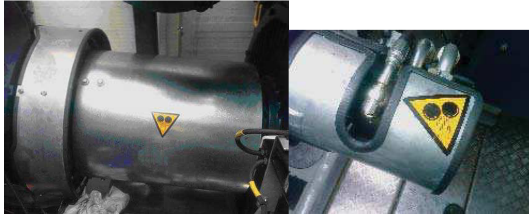
Figure 3.3.1: “Rotating Parts Behind” (item 208017) Place the sign on the cover for the composite coupling and on the cover for the rotating hydraulic union.
