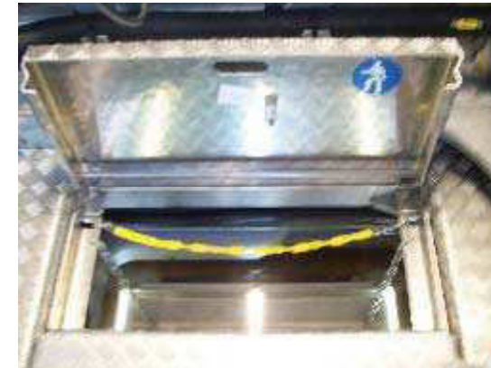
Figure 3.1: “Safety Harness Required” (item 208006) Place the sign underneath the rear door to the crane hatch.
