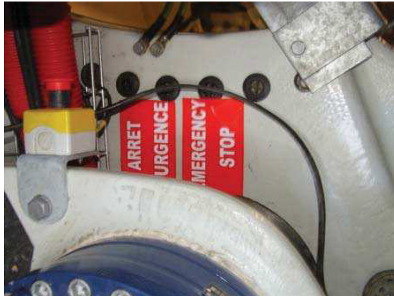
Figure 3.3.6: “Emergency Stop / Arrêt d’urgence” Place the sign under the gearbox next to the button
