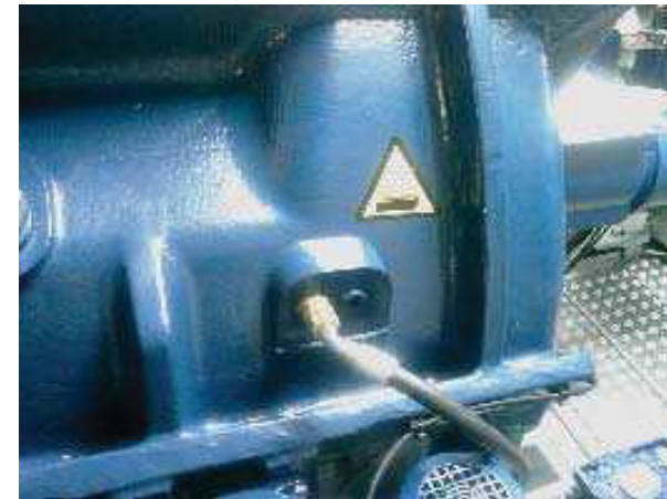
Figure 3.3.3: “Hot Surface” (item 208023) Place the sign on the left side of the gearbox.
