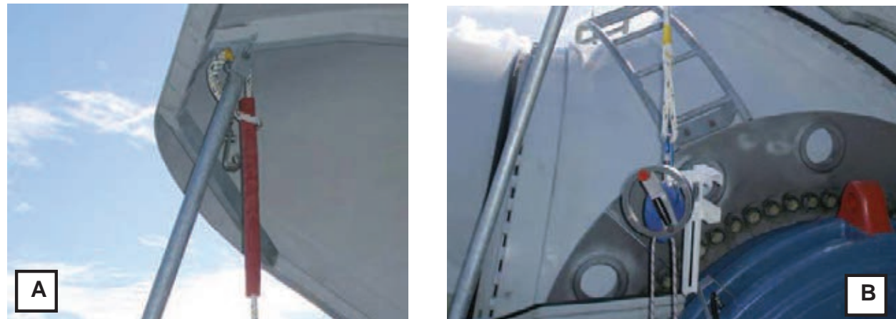
Fig. 30 Additional attachment point for the K08 beta turbine class
