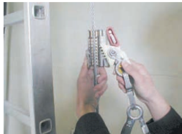
Fig. 13 Attaching the fall arrester to the safety rope
