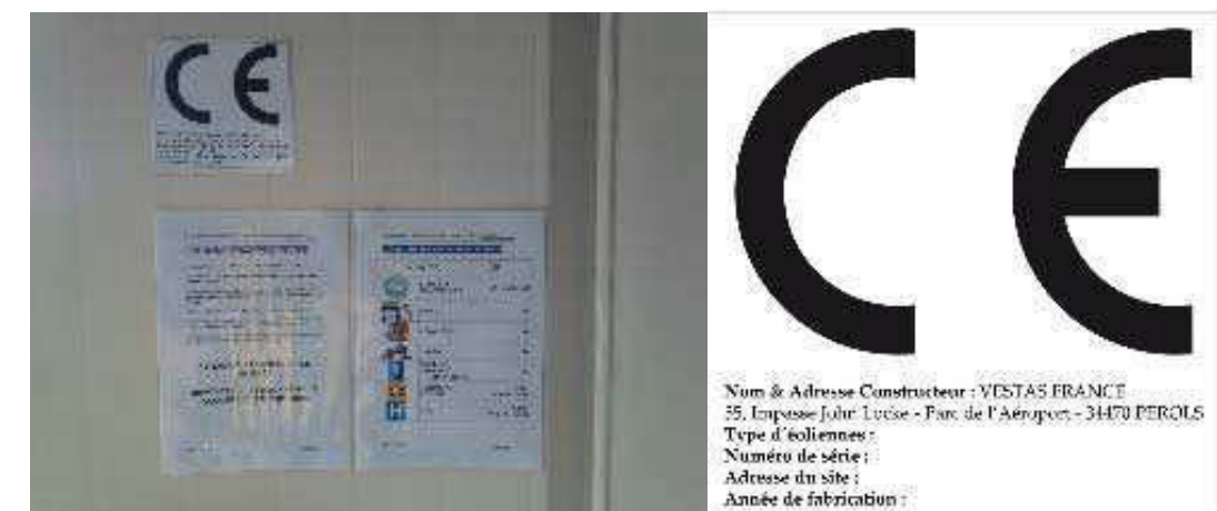
Figure 2.1.6: “Emergency Plan”, “CE mark” Place the signs on the bottom section at the right of the door
