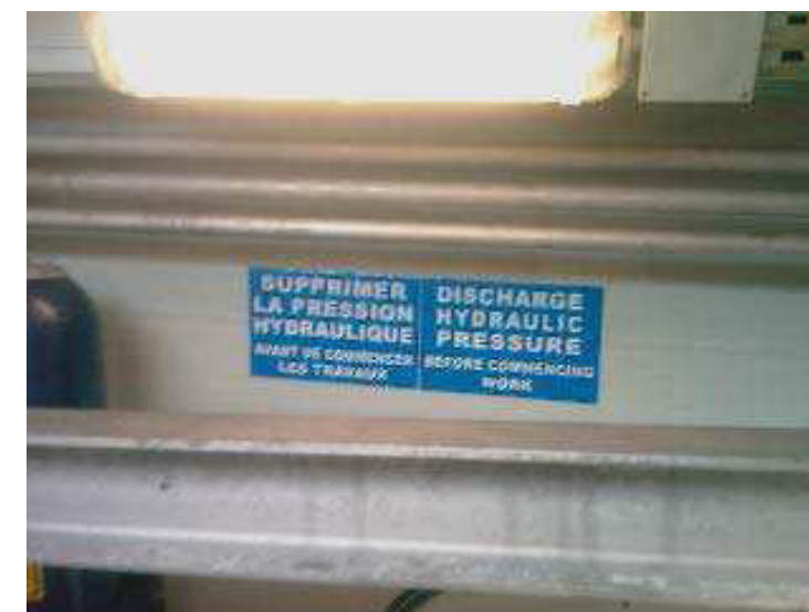
Figure 3.4.2: “Supprimer la pression hydraulique ... / Discharge hydraulic pressure” Place the signs near the hydraulic station
