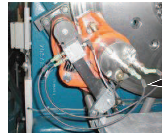
Fig. 58 Sensor for checking the brake pad thickness
