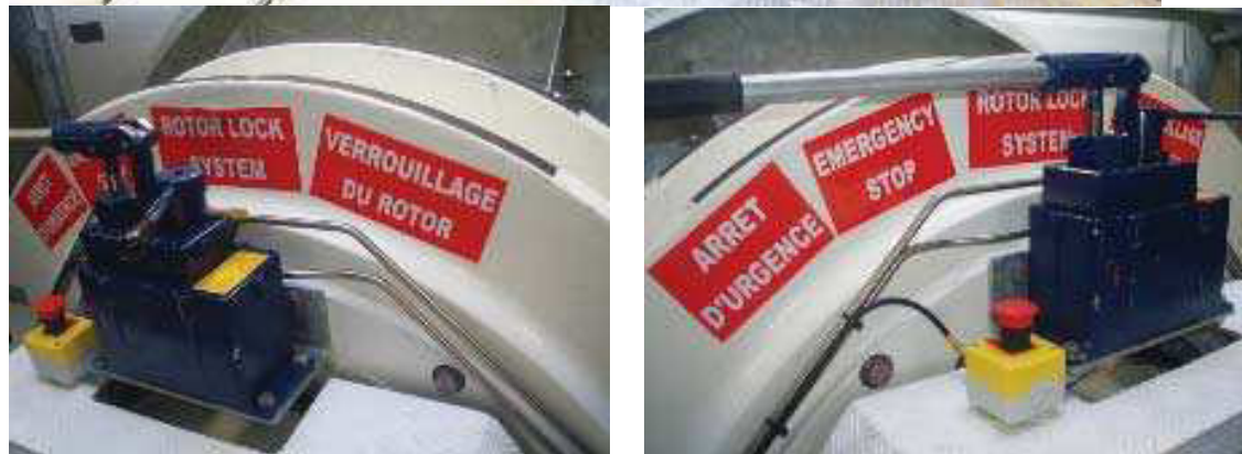
Figure 3.4.3: “Emergency Stop / Arrêt d’urgence”, “Rotor Lock System / Verrouillage du rotor” Place the signs around the parts
