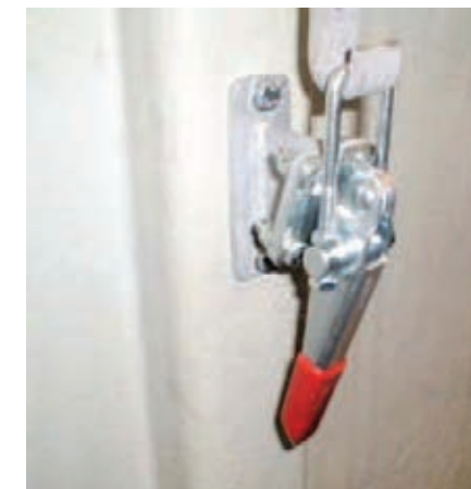
Fig. 36 Lock on the left nacelle wall
